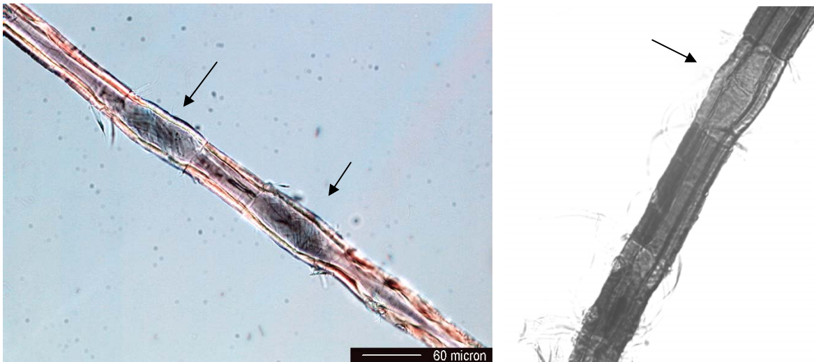
Figure 4.25. Light micrographs of wet TMP fibers showing fiber wall swelling where the outer wall layers have been removed (->).
