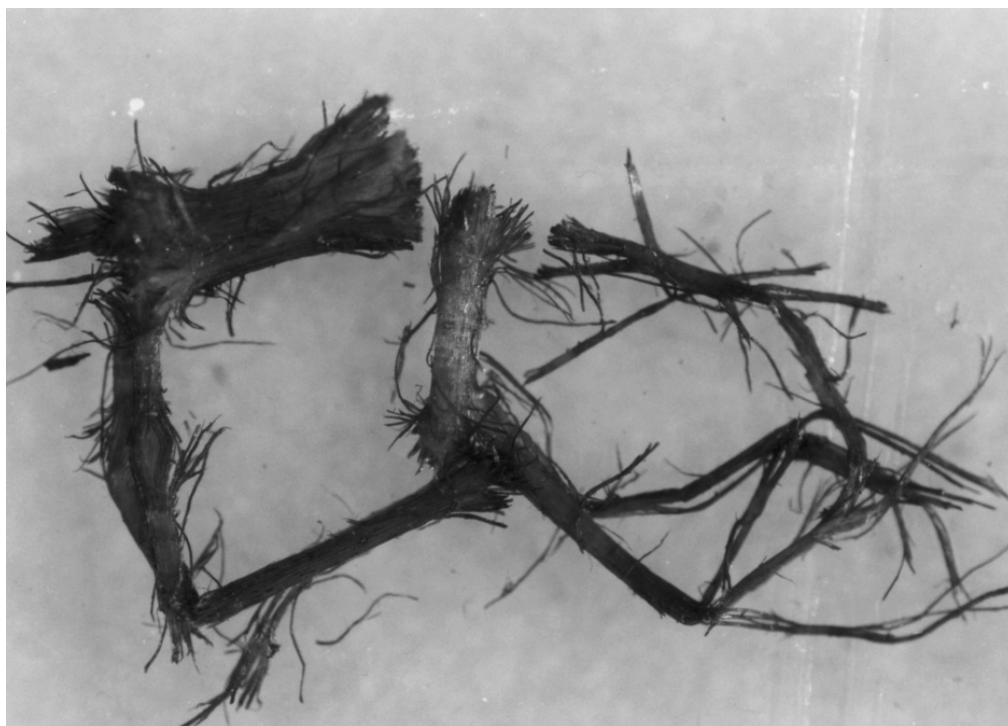
Figure 4.2 Undefibrated particles of RMP contained thick particles with broomed ends.
