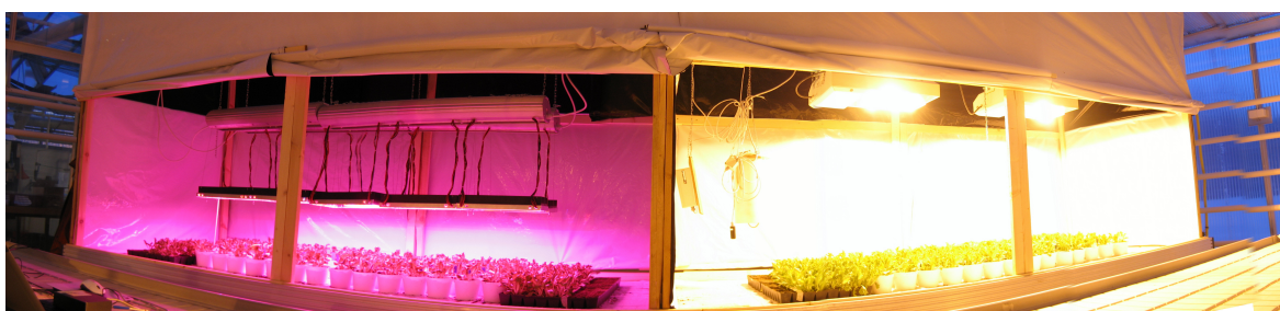
Figure 8 - Panoramic view of two of the growth blocks composed of LED luminaires (left) and high-pressure sodium luminaires (right) used in T2 test during week 2 on March 1 st 2006 at 7:29 AM. [IX]
