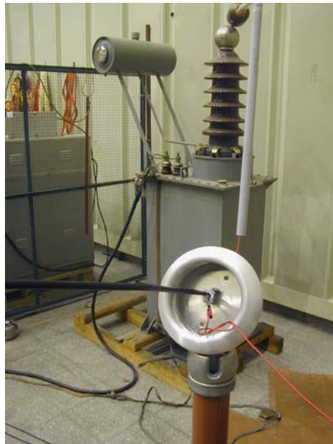
Fig. 3.7 Application of 20 kV AC supply for energizing conductor
