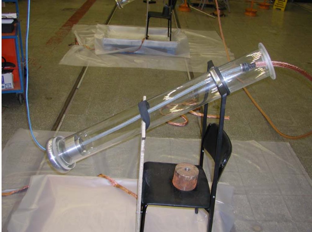
Figure 4.5 Oil-filled cable termination used during the breakdown testing.
