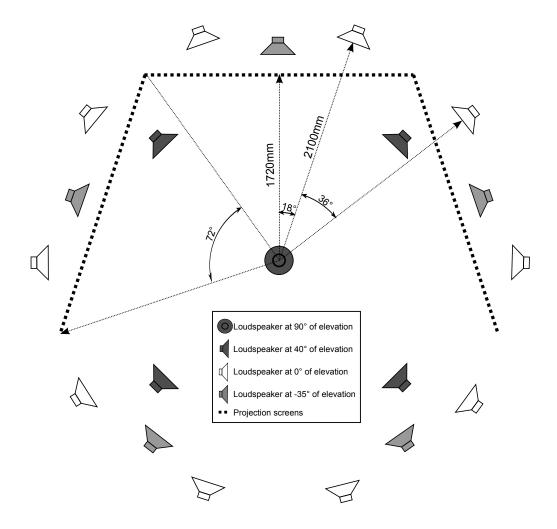
Figure 3.7: Loudspeaker layout of the deployed audiovisual environment. From [21].
