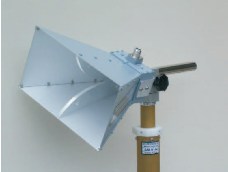
Figure 14: An example of a ridged horn antenna (Schwarzbeck BBHA 9120 D) [37].
