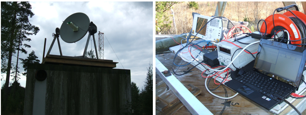
Figure 5.2: The steerable RFI-monitor system, log-periodic PCB antenna attached into parabolic dish (left), spectrum analyser, amplifier + voltage source and a laptop for harvesting the data (right).
