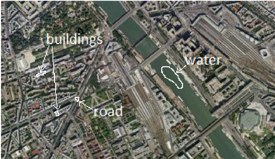
Figure 7: An example of training statistics collection from an optical image of Paris. Three classes exist, water, road and buildings, as do few samples for these classes. (Image source Microsoft Virtual Earth.)
