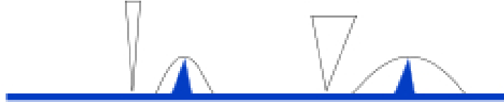
Figure 17: The effect of the size of the scanning tip in AFM on the resulting image. If the shape on the sample is sharper than the tip, the image will be determined by the size of the tip.
