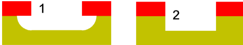
Figure 15: Typical etching patterns of isotropic (1) and anisotropic (2) etching.
