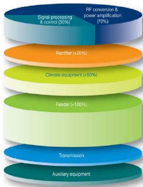
Figure 2: Energy consumption in a typical macro BS site [8]
