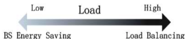
Figure 5: Relation between BS Energy Saving and Load Balancing [6]
