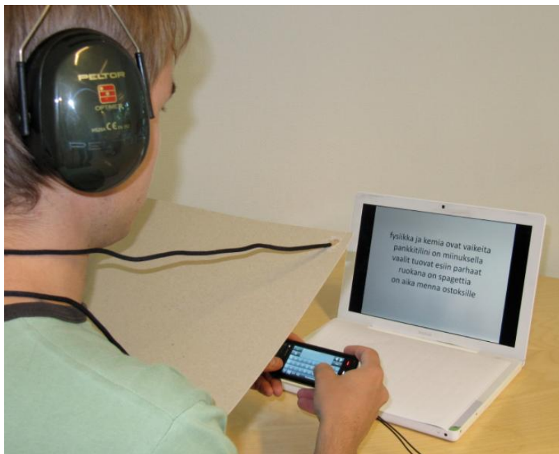
Figure 4. Tactile feedback unblocked and vision (cardboard) and audition (ear protection) blocked.
