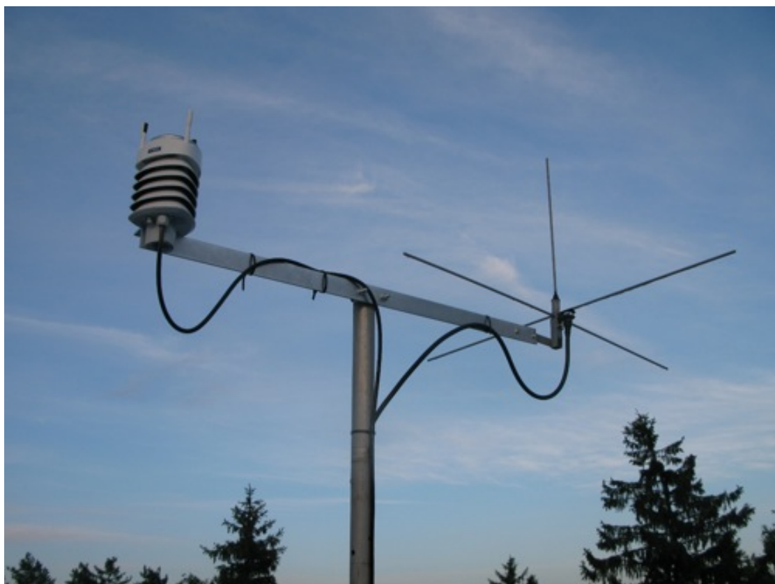
Figure 7.1: AWS installed to simulate a real scenario.
