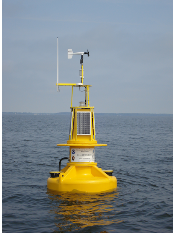
Figure 3.1: NOAA weather buoy [32], example of a complex and robustness AWS.
