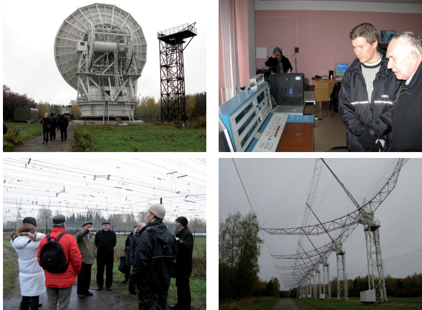
Figure 7.1. The XI Russian-Finnish Astronomy Symposium. First row, left: The 22-metre radio telescope RT22. Right: RT22 control room. Second row, left: Large Phased Array, operating in the metre-wavelength range. Right: Wide-band Cross Type Array DKR-1000.
