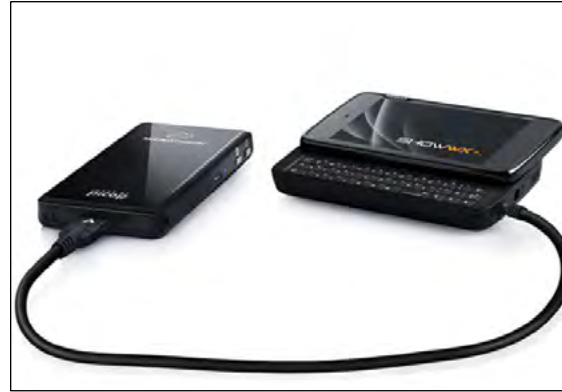
Figure 3: Pico projector connected to a phone (Microvision)
