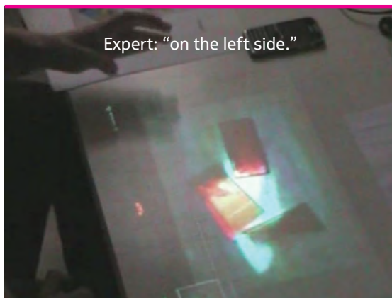
Figure 56: Non-transmitted gesture (user does not realize his hand is not seen or is not aware that he can use his gestures for interaction).
