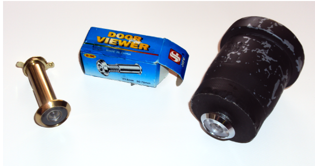
Figure 20: A DIY fisheye lens
