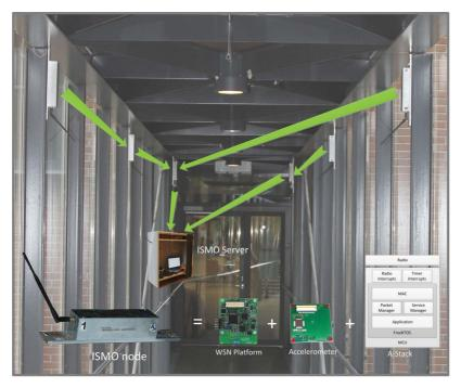
Figure 6.8. Structural health monitoring system deployment on a footbridge using A-Stack
