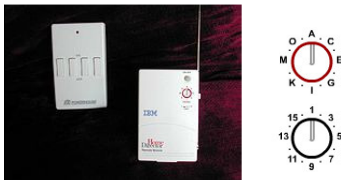
Fig 2.1. A typical 4-channel radio switch and radio-to-power line transponder (left) and X-10 controllers [6]
