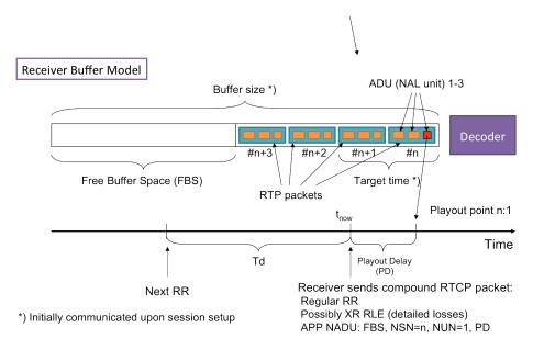
Figure 20: Receiver Side Model for NADU
