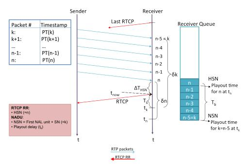
Figure 28: Time Since Receiving Last Packet ( $\Delta T_{HSN}$ )
