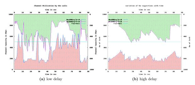
Figure 40: Plot of Goodput of two VVoIP streams sharing a common bottleneck link of 1Mbps.
