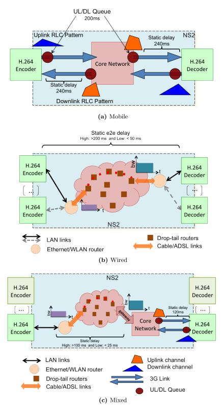
Figure 23: shows the (a) 3G, b) wired Internet (c) mixed simulation environment
