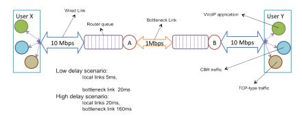
Figure 37: Simulation setup for comparing dissimilar traffic
