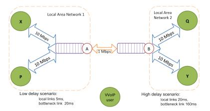
Figure 39: Simulator representation and setup
