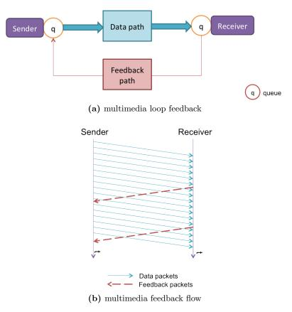
Figure 7: Feedback loop and Feedback timing
