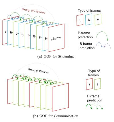
Figure 3: shows the typical Group of Pictures (GOP) arrangement for (a) Video Streaming (b) Video Communication
