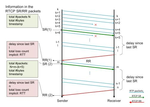
Figure 14: RTP and RTCP Flow Diagram
