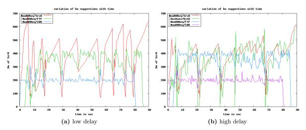
**Figure 38:** Plot of Application bit rates for a VVoIP stream, TCP and UDP sharing a common link of 1Mbps.
