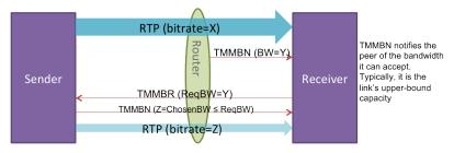
Figure 18: RTCP header extension for TMMBR/TMMBN specified in Codec Control Message
