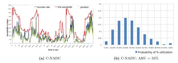
Figure 35: Plot of Link rate, encoder rate, goodput (left column) and Histogram of Probability of per-instance %Utilization (right column) and Average BW Utilization (ABU) of Dynamic 3G Links by C-NADU
