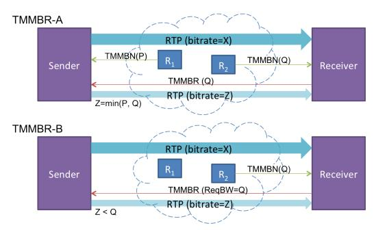
Figure 31: Operating model for TMMBR-A, and TMMBR-B
