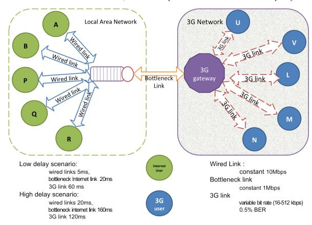
Figure 42: Mixed or heterogeneous simulation setup
