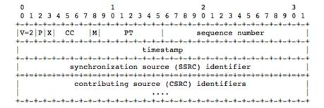
Figure 13: Block representation of a basic RTP Packet
