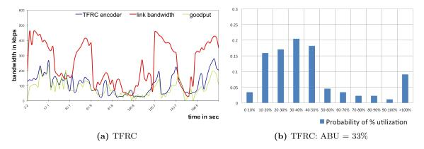
Figure 33: Plot of Link rate, encoder rate, goodput (left column) and Histogram of Probability of per-instance %Utilization (right column) and Average BW Utilization (ABU) of Dynamic 3G Links by TFRC
