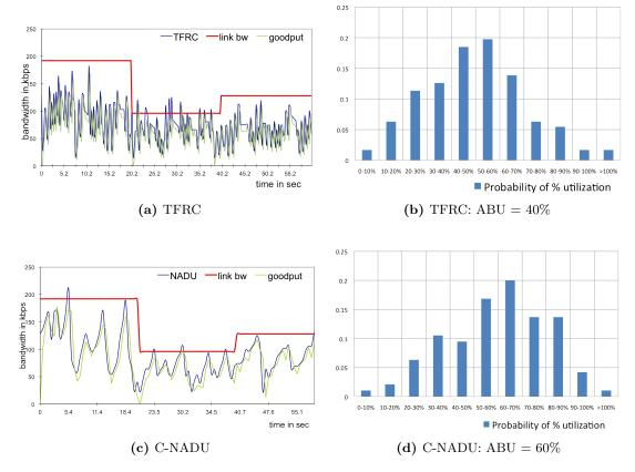
Figure 36: Plot of Link rate, encoder rate, goodput and Histogram of Probability of per-instance %Utilization (right column) and Average BW Utilization (ABU) in stable and slowly varying bandwidth scenario.
