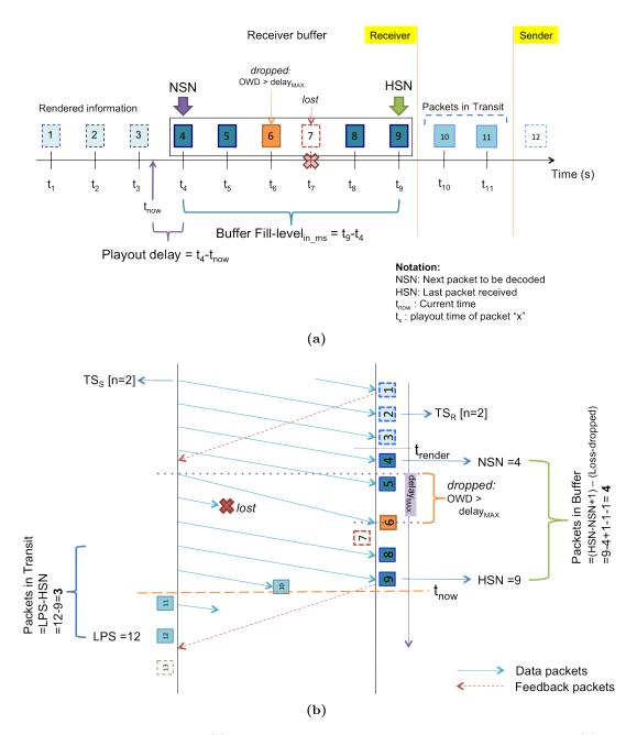
**Figure 9:** Visualization of the (a) Decoder Timeline during an ongoing VVoIP call, and (b) flow of packets. Both figures describe calculation of congestion indicators
