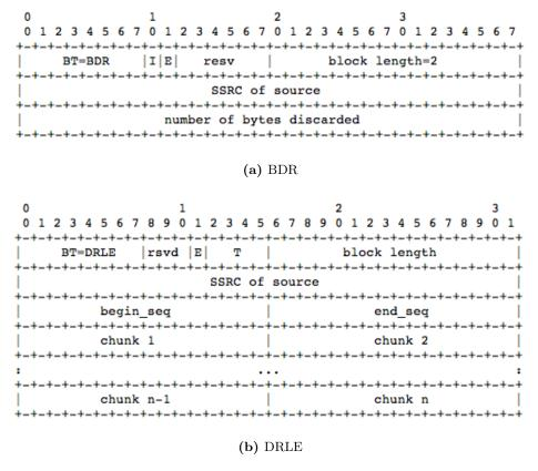
Figure 26: RTCP header extension for signaling the (a) bytes discarded per RTCP interval during a multimedia session, (b) discarded packet pattern at the receiver
