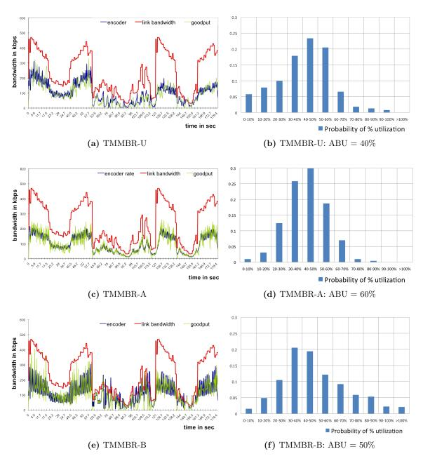
Figure 34: Plot of Link rate, encoder rate, goodput (left column) and Histogram of Probability of per-instance %Utilization (right column) and Average BW Utilization (ABU) of Dynamic 3G Links by (a) TMMBR, (b)TMMBR-A, (c)TMMBR-B
