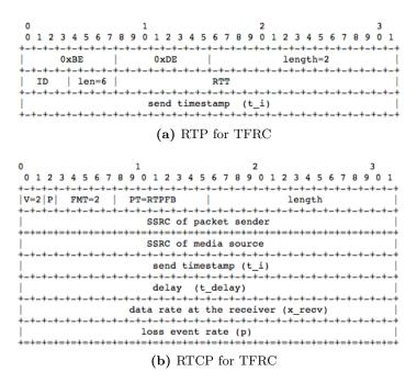
**Figure 17:** TFRC adapted for multimedia sessions: (a) RTP header extension (RTP/TFRC), (b) RTCP extension (TFRC-FB)
