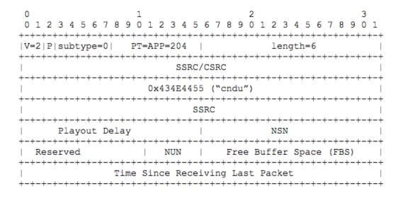
Figure 29: RTCP header extension for C-NADU
