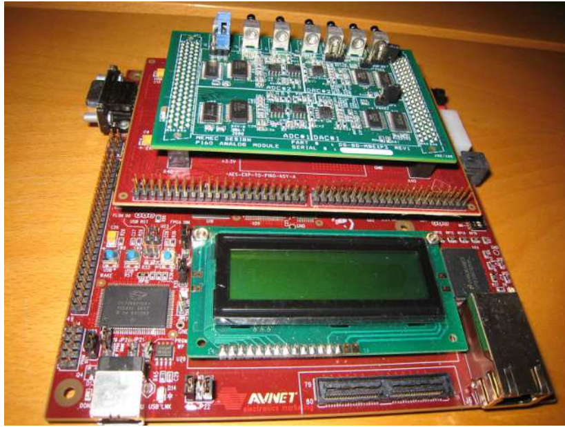
Figure 5.2: Avnet Xilinx Virtex-5 LX50 evaluation board with expansion modules.
