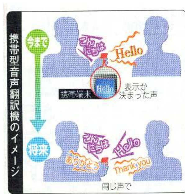
Figure 1.1: The EMIME system, pictured below, changes the "colour" of the synthesised voice to match the current user. An improvement over the old systems, above, that always use the same synthesised voice. From Mainichi Newspaper, May 20th 2008.
