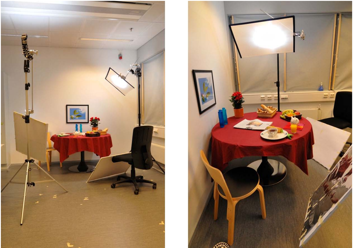
Figure 14. The lighting setup of Reference Image II, illustrating the placement of two flash units and two reflector plates.
