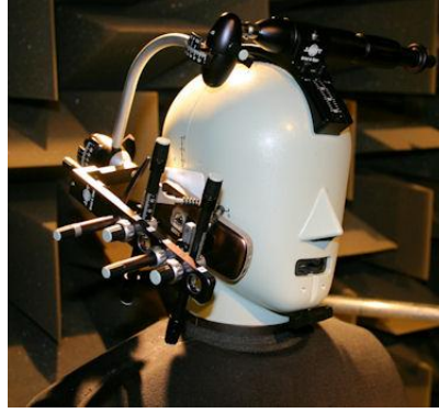
Figure 28: Nokia 6720 classic positioned to 3GPP measurements HATS in anechoic chamber.
