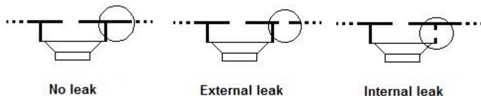
Figure 18: Different leak types used in mobile phone earpiece enclosure [31].
