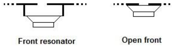
Figure 16: Different mobile phone earpiece front realizations [31].
