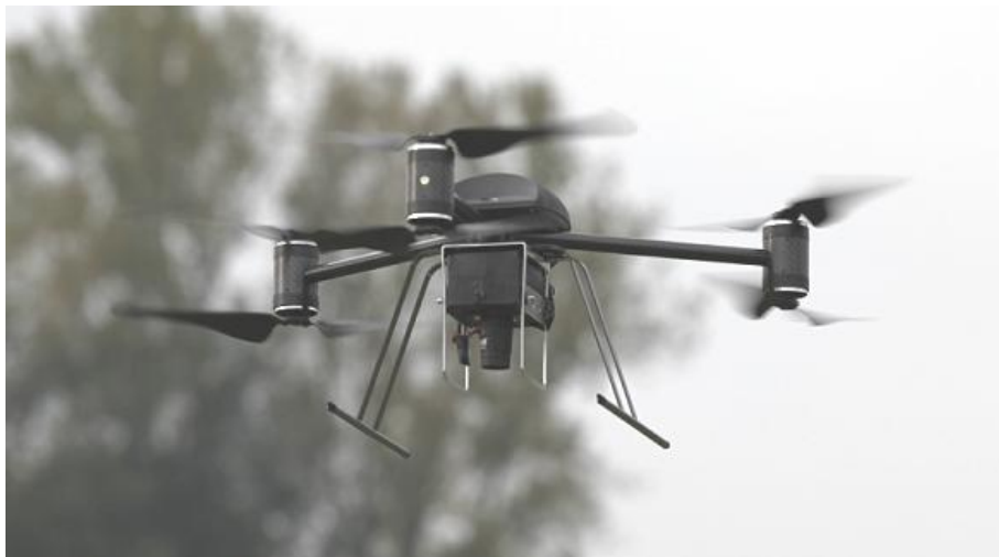
Figure 9.1. The hyperspectral imager was mounted on a UAV helicopter for test flights. The mass of the hyperspectral imager including the battery is 350g so it can be easily carried by the helicopter.
