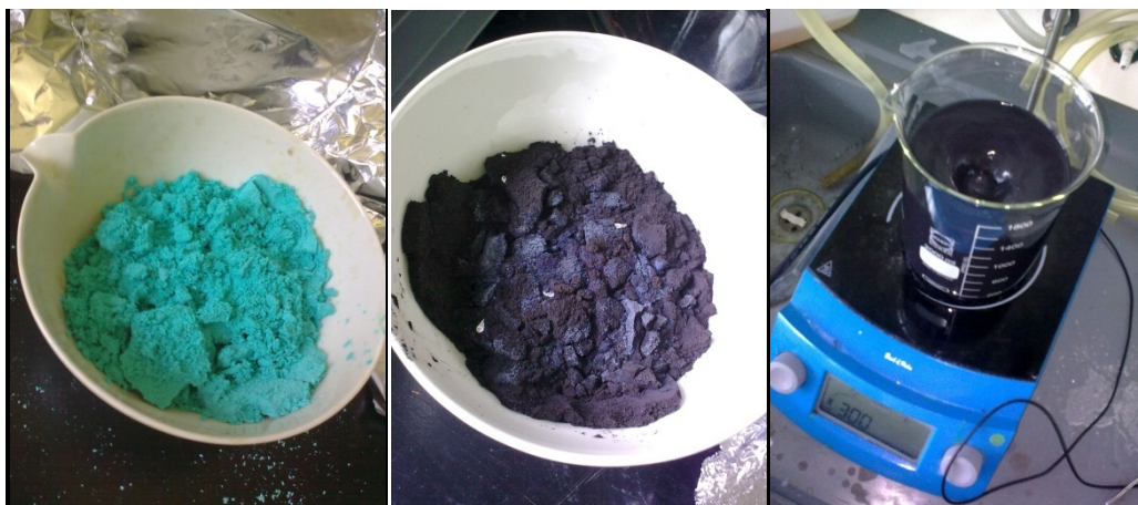
Figure 13: Catalyst production. Left and middle: before and after calcination in oven. Right: stirring the catalyst in 0.5 wt% \text{NH}_4\text{HCO}_3 solution.
