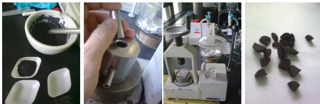
Figure 14: Catalyst tablet preparation.
