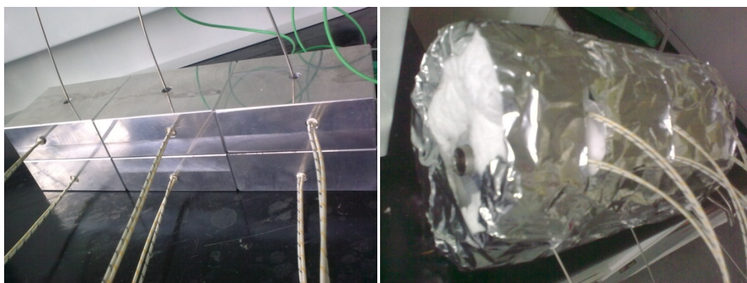
Figure 10: Left: Evaporator/Reformer unit with three thermocouples going in from the top and six heating cartridges going in from the side. Right: The unit is heat insulated with mineral wool and covered with aluminium foil for more convenient handling.
