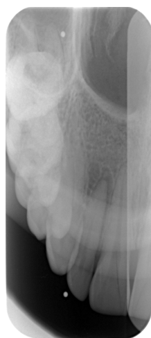
Figure 12: Sample image of the imaging plate showing a distinct vertical border—or change in the overall gray levels—on the right side of the image. It has been caused by another imaging plate on top this one during the exposure.
