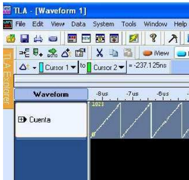
Figure 4.17: Logic analyzer capture of a 10-bit ramp
