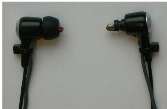
Figure 4.4: A pair of Philips earphones with mounted in-ear microphones [17]. The headphones are similar except that the rubber ear cap of the right-hand side headphone has been removed in order to bring out the in-ear microphone.
