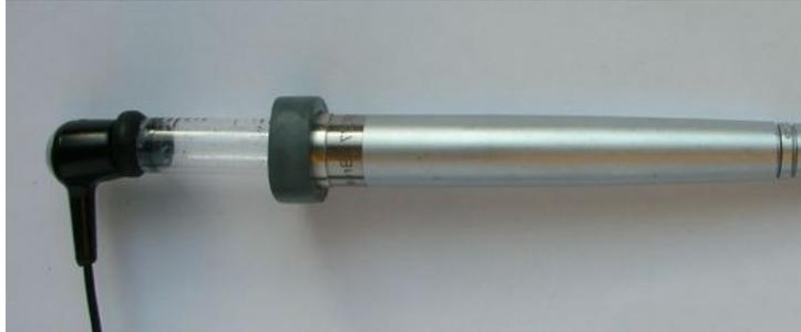
Figure 4.5: Headphone adapter attached for Brüel&Kjær's 4191 Microphone.
