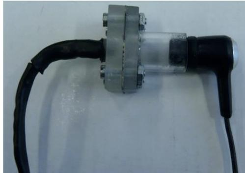
Figure 4.1: The headphone (on the right) and the Sennheiser KE-4 microphone (on the left) are attached to the simple ear canal simulator (in the middle) [30].
