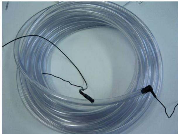
Figure 4.3: The resistive-load tube
