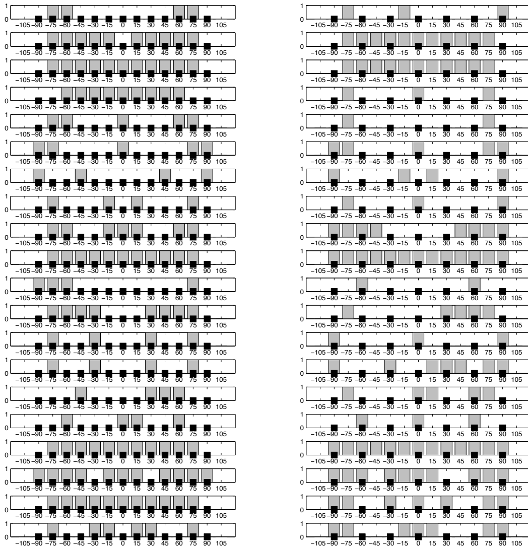
Figure 6.5: Results of cases 7 (left) and 14 (right). All 20 answers are plotted. The numbers from -105 to 105 indicate the angles in which the loudspeakers were. Black boxes indicate the loudspeaker that were emitting sound. The grey bars indicate that the particular loudspeaker was marked as emitting sound.
