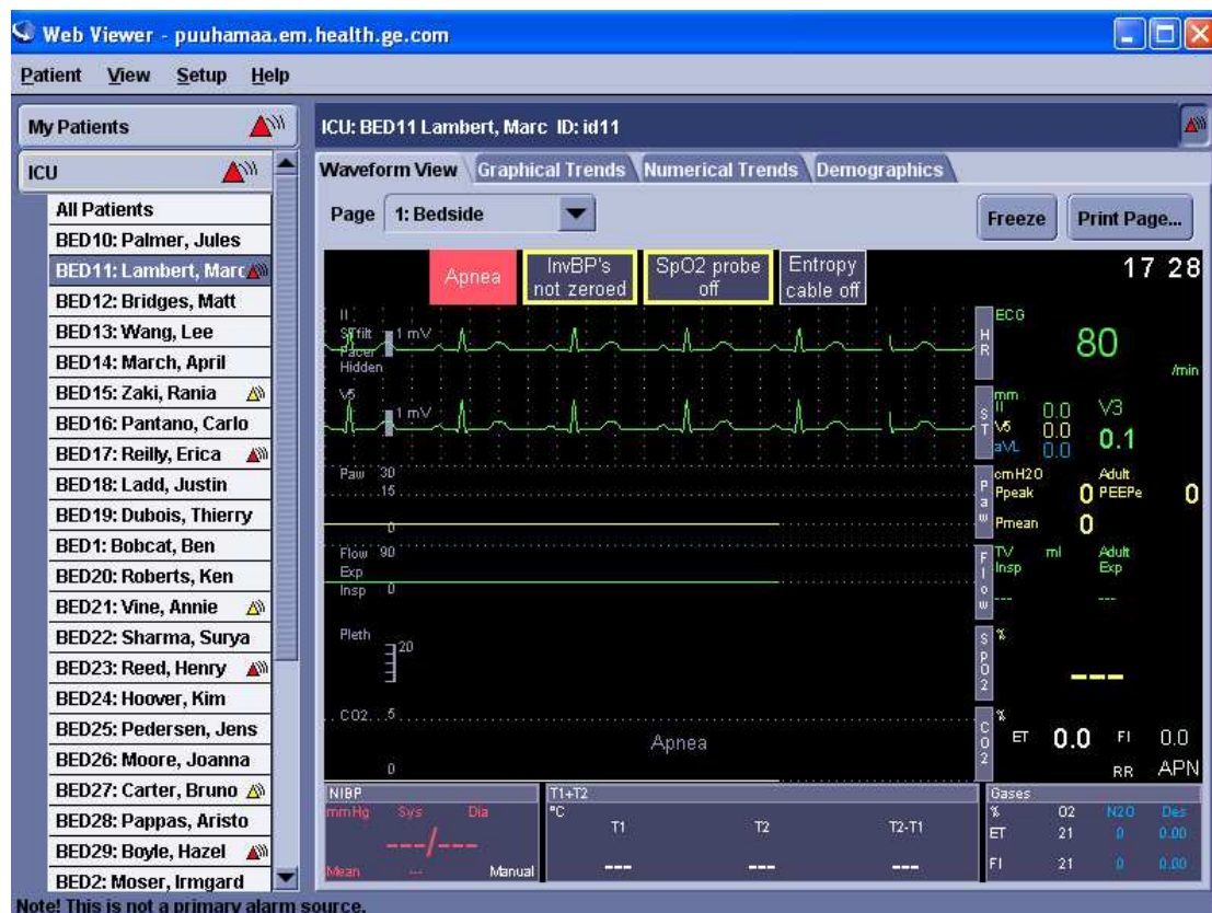
Figure 2 Web Viewer client application
