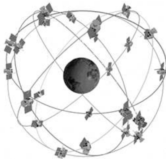
Figure 2.16: The 24 satellites orbiting the earth at the altitude of 11 000 nautical miles provide global position tracking around the globe. [30]
