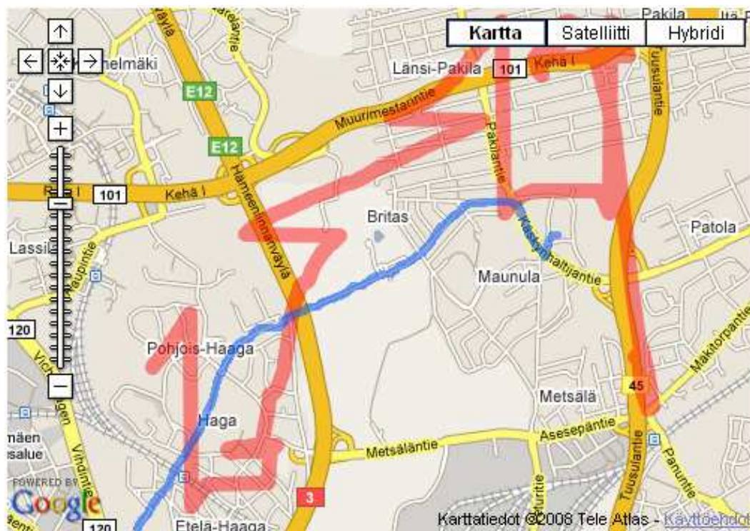
Figure 6.3: The positioning does not work properly unless the signal from at least three satellites is received. The recording was done while sitting in a bus. The red line represents the recorded path and the blue line the actual path.
