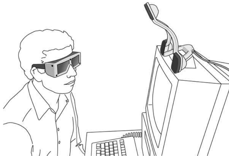
Figure 2.13: Logitech 3D Head Tracker. The triangle-shaped transmitter with three ultrasonic speakers at the corners is positioned on top of the monitor. Three microphones to receive the signals are located in this case in the 3D-glasses worn by the user. [28]
