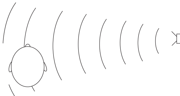
Figure 2.5: Interaural Level Difference – ILD
