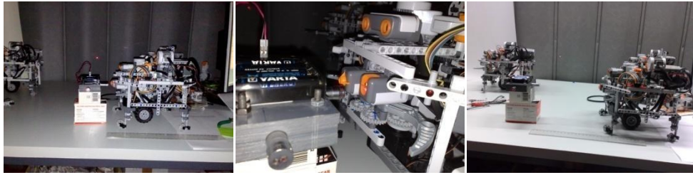
Fig. 35. The start condition seen from the side of both units (left), a close-up of the laser pointer being 1 cm in front of the light sensor (center), and the end condition of both units 20 cms from each other (right) while performing the test 5.1.10. in dark room conditions.
