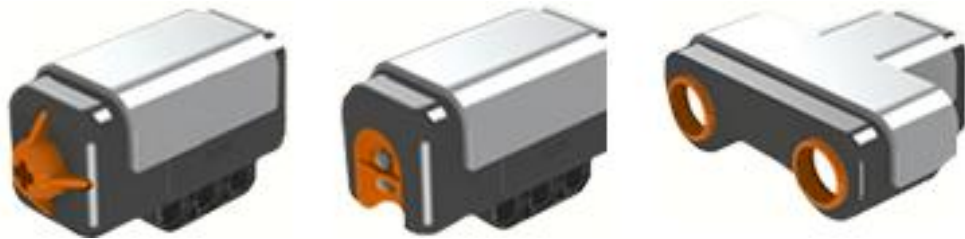
Fig. 14. From left to right touch, light and ultrasonic NXT sensors.
