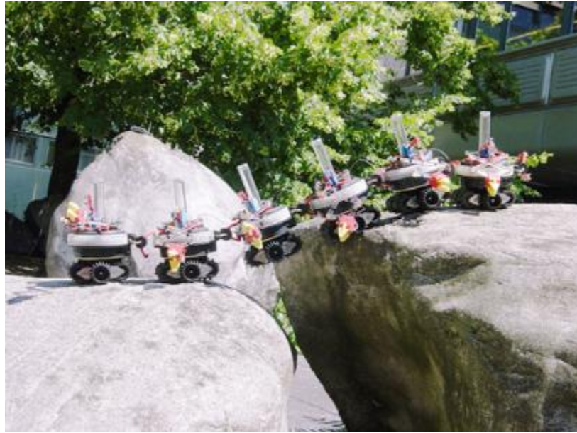
Fig. 10. Swarm-Bot going over a big gap.
