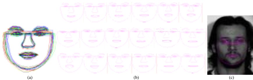
Figure 5.9. Example of facial feature extraction and representation by ASM: (a) aligned training set of facial features, (b) the first three modes of the model, (c) searching result.
