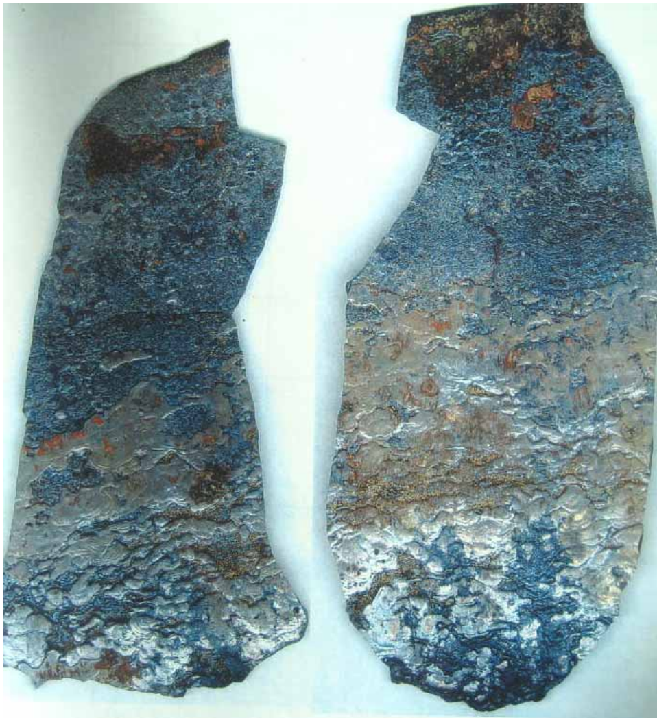
Figure 16 . An example of surfaces of slag layers on the mould side; cast number 80330. Height of sample is approximately 25cm and the upper edge is a few centimeters below the meniscus.
