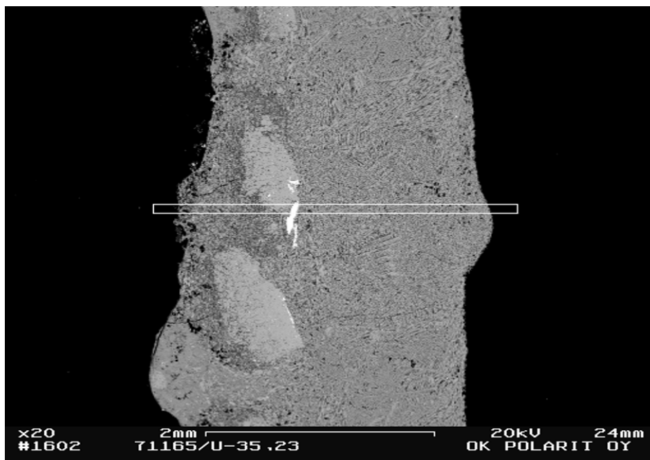
Figure a9. Layer on outer bow side 23 cm from meniscus.
