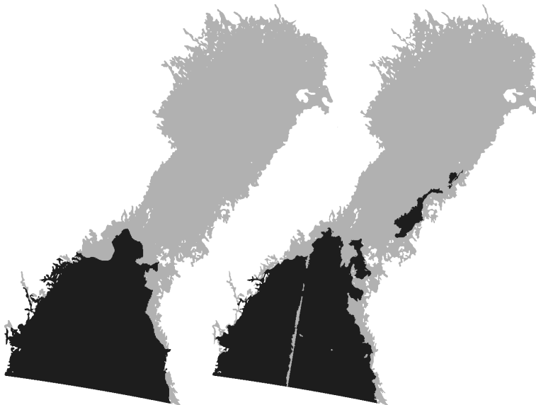
Figure 7.5: Open sea (darker gray tone) and ice in the area of the SAR image in Fig. 7.4 according to the ice chart, left. Open sea and ice in the area of the SAR image in Fig. 7.4 according to our algorithm, right.
