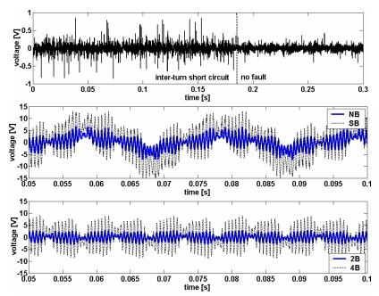
Fig. 5.2.7 Time-domain representation of the voltages induced in search coil "p-1" – interturn short circuit – measurements (topmost figure) and simulations taken at half load.
