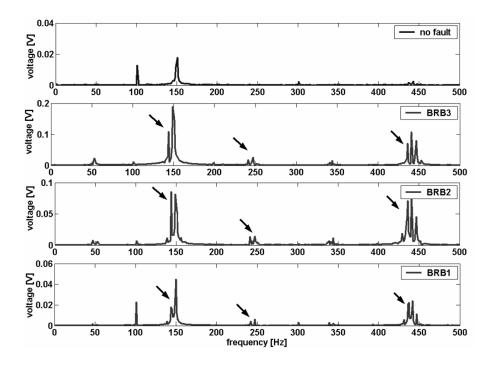
Fig. 5.2.28.a Frequency-domain representation of the voltages induced in search coil "p+1" during various cage-related faults – measurements at full load.
