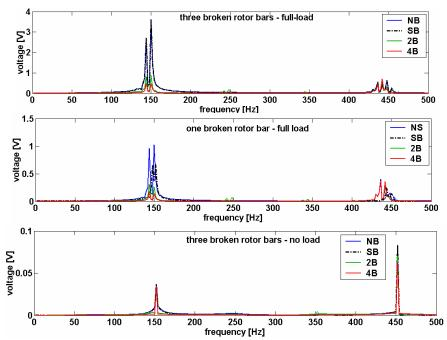
Fig. 5.2.27 Frequency-domain representation of the voltages induced in the "p+1" search coil during various cage-related faults – simulations at various loads.
