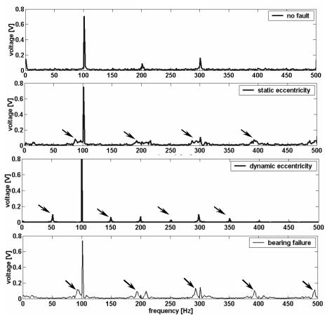
Figs. 5.3.23 Frequency-domain representation of the voltages induced in a search coil placed around the motor shaft – static eccentricity, dynamic eccentricity, bearing fault – measurements at half load.
