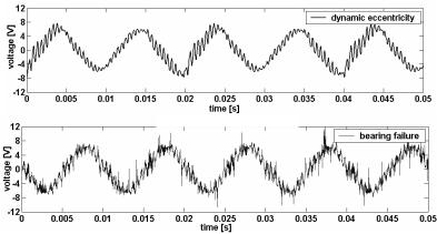
*Fig. 5.3.1 Time-domain representation of the voltages induced in the search coil placed around a stator tooth – bearing failure, dynamic eccentricity – measurements at half load.*
