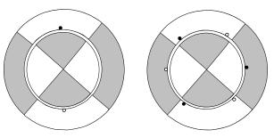
*a)* search coil "p-1" *b)* search coil "p+1" Fig. 3.5 Search coils positioning for measuring the " $p\pm 1$ " harmonics (the test motor has p=2).
