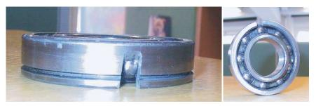
Fig. 2.5 Artificially created bearing fault studied in this work.
