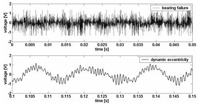
*Fig. 5.3.6 Time-domain representation of the voltages induced in the search coil placed around two pole pitches – bearing fault, dynamic eccentricity – measurements at half load.*
