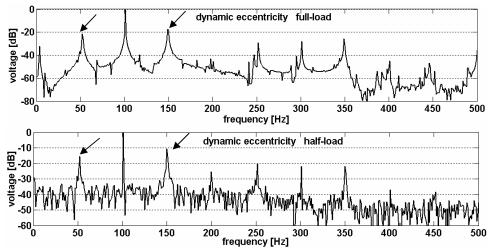
*Fig. 5.3.8 Frequency-domain representation of the voltages induced in a search coil placed around two pole pitches – dynamic eccentricity – measurements at various loads.*
