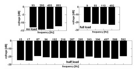
*Fig. 5.3.25 Characteristic frequency sideband components produced by the static eccentricity in the indications provided by the search coil wound around the motor shaft – measurements.*
