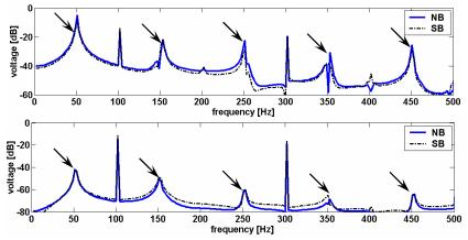
Fig. 5.2.9 Characteristic frequency sidebands produced by the inter-turn short circuit in the indications provided by "p-1" search coil – simulations at full load (top) and no load (bottom).
