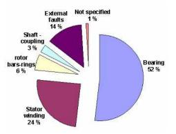
Fig. 2.2 Distribution of failures among failed components for electrical machines working in the petrochemical industry (Thorsen and Dalva 1999).
