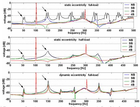
*Fig. 5.3.4 Frequency-domain representation of the voltages induced in the search coil placed around a stator tooth – simulations at various loads.*
