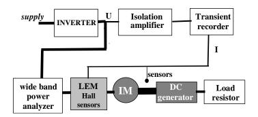
Fig. 4.5 Schematic of the measuring set-up.
