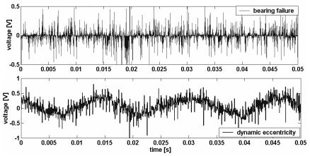
*Fig. 5.3.22 Time-domain representation of the voltages induced in the search coil positioned at the non-drive end of the motor – bearing fault, dynamic eccentricity – measurements at half-load.*
