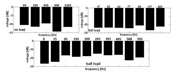
Fig. 5.3.26 Characteristic frequency sideband components produced by bearing fault in the indications provided by the search coil wound around the motor shaft – measurements at various loads.
