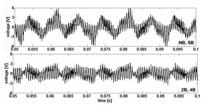
Fig. 5.3.18.b Time-domain representation of the voltages induced in search coil "p-1" – dynamic eccentricity – simulations at half load.
