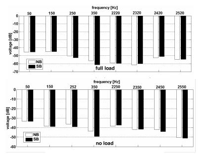
Fig. 5.3.10 Characteristic frequency sidebands produced by static eccentricity in the indications provided by the search coil placed around two pole pitches of the test motor – simulations at various loads.
