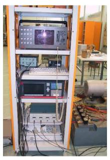
*Fig. 4.7 Measurement devices. From top to bottom: transient recorder, keyboard, power analyser, isolation amplifier, and connection box.*
