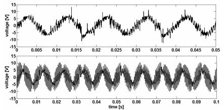
Fig. 5.2.16 Time-domain representation of the voltages induced in the search coils placed around stator tooth -3 broken rotor bars - measurements (top) and simulations (bottom) taken at half load.
