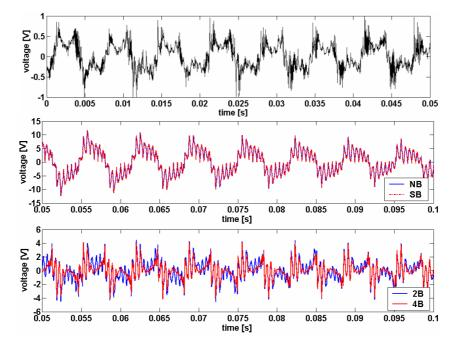
Fig. 5.2.26 Time-domain representation of the voltages induced in the search coil "p+1" – three broken rotor bars – measurements (top) and simulations at half load.
