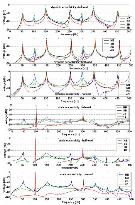
*Fig. 5.3.9 Frequency-domain representation of the voltages induced in the search coil placed around two pole pitches – static eccentricity, dynamic eccentricity – simulations at various loads.*
