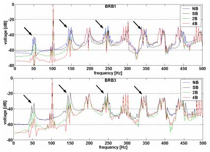
Fig. 5.2.18 Frequency-domain representation of the voltages induced in the search coil wound around a stator tooth -1 broken rotor bar (top) and 3 broken rotor bars (bottom) - simulations taken at half load.
