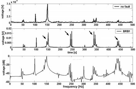
Fig. 5.2.25.a Frequency-domain representation of the voltages induced in the "p-1" search coil – one broken rotor bar – measurements at full load.
