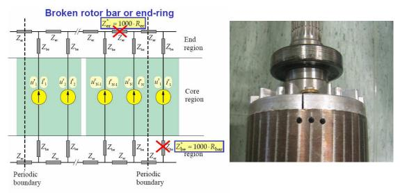
*Fig. 4.3 Description of the rotor cage-related faults implemented in simulations (left figure) and artificially created in measurements (right figure).*
