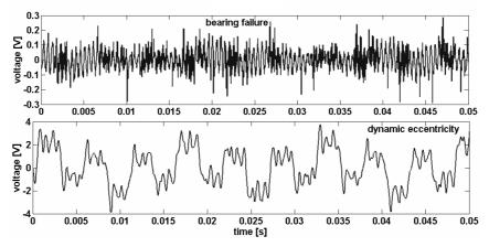
Fig. 5.3.17 Time-domain representation of the voltages induced in search coil "p-1" – bearing fault, dynamic eccentricity – measurements at half load.
