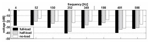
Fig. 5.3.27 Characteristic frequency sideband components produced by the dynamic eccentricity in the indications provided by the search coil wound around the motor shaft – measurements at various loads.
