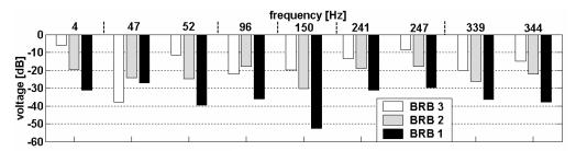
Fig. 5.2.31 Characteristic frequency sidebands produced by various rotor cage-related faults in the indications provided by the search coil placed around the motor shaft – measurements at full load.
