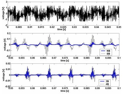
*Fig.* 5.2.5 *Time-domain representation of the voltages induced in the search coil placed around two pole pitches of the test motor – inter-turn short circuit – measurements (topmost figure) and simulations taken at half load.*
