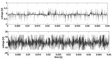
*Fig. 5.2.29 Time-domain representation of the voltages induced during a cage-related fault in the search coils located at the non-drive end of the motor near the ventilator (top) and around the motor shaft (bottom) – measurements at full load.*
