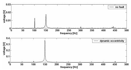
Fig. 5.3.15 Frequency-domain representation of the voltage induced in the "p+1" search coil – dynamic eccentricity – measurements at full load.
