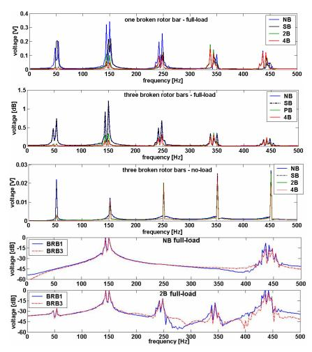
*Fig. 5.2.24 Frequency-domain representation of the voltages induced in the "p-1" search coil during various cage-related faults – simulations at various loads.*
