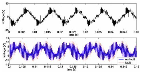
*Fig. 5.2.1 Time-domain representation of the voltages induced in the search coil placed around stator tooth – inter-turn short circuit in the stator winding – measurements (top) and simulations (bottom) taken at half load.*
