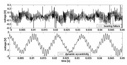
Fig. 5.3.11 Time-domain representation of the voltages induced in search coil "p+1" – bearing fault, dynamic eccentricity – measurements at half load.
