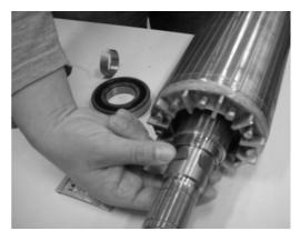
Fig. 4.2 Artificially created dynamic eccentricity.
