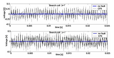
*Fig. 5.4.1 Time-domain representation of the voltages induced in the* "p-1" (top) and "p+1" (bottom) search coils in motor operation with a core fault – simulations.
