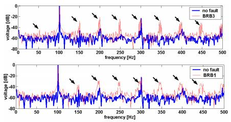
Fig. 5.2.17 Frequency-domain representation of the voltages induced in the search coil around stator tooth during rotor cage-related faults -3 broken rotor bars (top) and 1 broken rotor bar (bottom) – measurements at half load.
