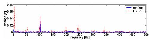
Fig. 5.2.21 Frequency-domain representation of the voltages induced in the search coil wound around two pole pitches -3 broken rotor bars - measurements at full load.
