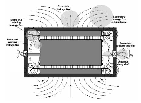
Fig. 3.3 Schematic of flux regions used for fault detection and condition monitoring of electrical machines (Thomson 1999).
