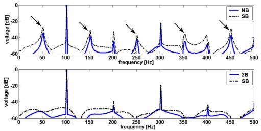
*Fig. 5.2.3 Frequency-domain representation of the voltages induced in the search coil wound around a stator tooth during the inter-turn short circuit – simulations at half load.*
