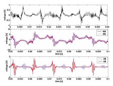
Fig. 5.2.23 Time-domain representation of the voltages induced in the search coil "p-1" – 3 broken rotor bars – measurements (top) and simulations taken at half load.
