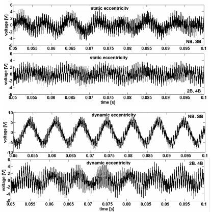
Fig. 5.3.12 Time-domain representation of the voltages induced in search coil "p+1" – static eccentricity, dynamic eccentricity – simulations at half load.
