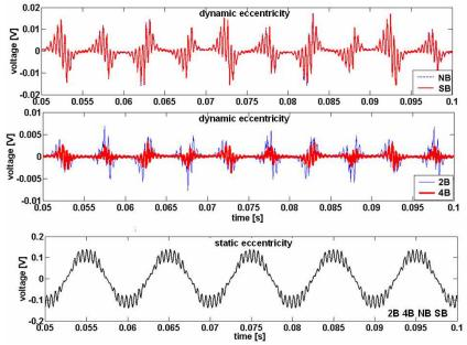
*Fig. 5.3.7 Time-domain representation of the voltages induced in the search coil placed around two pole pitches – simulations at half load.*
