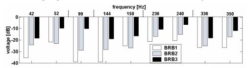
*Fig. 5.2.22 Characteristic frequency sidebands produced by various rotor cage-related faults in the indications provided by the search coil placed around two pole pitches – measurements at full load.*
