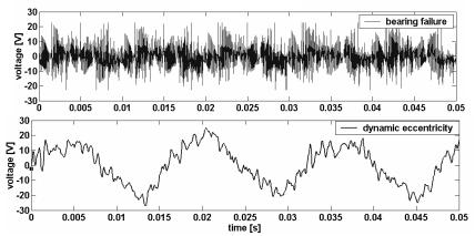
*Fig. 5.3.21 Time-domain representation of the voltages induced in the search coil located around the shaft – bearing fault, dynamic eccentricity – measurements at half-load.*
