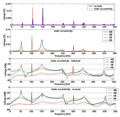
Fig. 5.3.19 Frequency-domain representation of the voltages induced in the "p-1" search coil – healthy and static eccentricity – measurements (topmost figure) and simulations with various loads.
