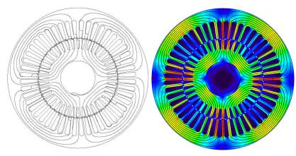
*Fig. 4.8 Cross-sectional geometry of the test motor and the electromagnetic field distribution for healthy operation at rated load.*
