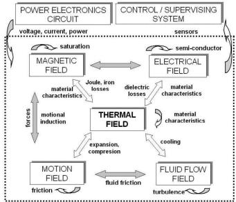
Fig. 3.1 Interactions of physical phenomena characteristic for a general electromagnetic energy converter structure (Driesen 2000).
