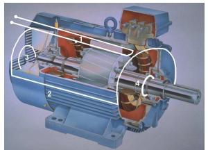
Fig. 3.4 Search coils used for the electromagnetic flux monitoring.
