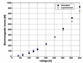
Fig. 5.1 Experimental and simulated total electromagnetic losses.
