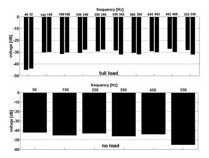
*Fig. 5.3.5 Characteristic frequency sidebands produced by static eccentricity in the indications provided by the search coil placed around a stator tooth – simulations.*
