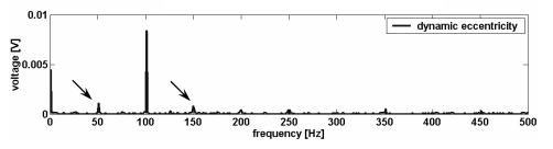
*Fig. 5.3.24 Frequency-domain representation of the voltage induced in a search coil placed at the non-drive end of the test motor – dynamic eccentricity – measurements at half load.*
