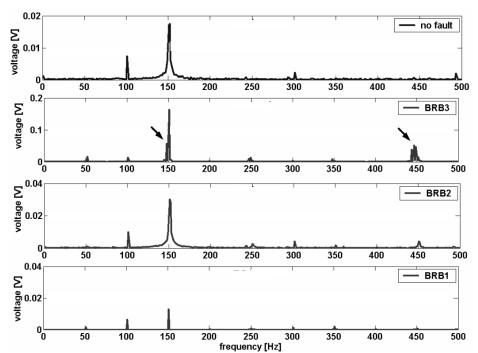
Fig. 5.2.28.b Frequency-domain representation of the voltages induced in search coil "p+1" during various cage-related faults – measurements at no load.
