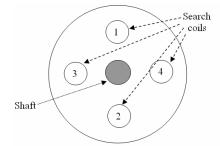
Fig. 3.6 Coil geometry arrangement for reliable turn fault location (Penman et al. 1994).
