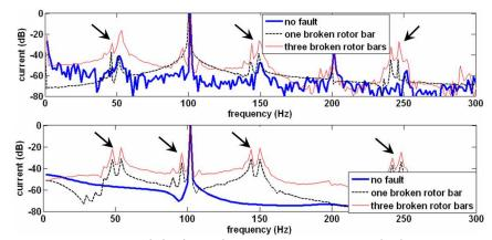
*Fig. 5.1.3 Frequency spectra of the branch current – rotor cage faults – measurements (top) and simulations (bottom) at full load.*
