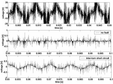
Fig. 5.2.14 Time-domain representation of the voltages induced during the inter-turn short circuit in search coils positioned around the motor shaft and at the non-drive end of the motor (topmost figure) – measurements at half load.
