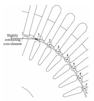
Fig. 4.4 Description of the core fault implemented in the simulations.
