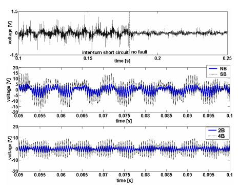
Fig. 5.2.10 Time-domain representation of the voltages induced in search coil "p+1" during the inter-turn short circuit – measurements (topmost figure) and simulations taken at half load.
