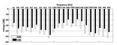
Fig. 5.2.4 Characteristic frequency sidebands produced by the inter-turn short circuit in the indications provided by a search coil wound around a stator tooth – simulations at full load.
