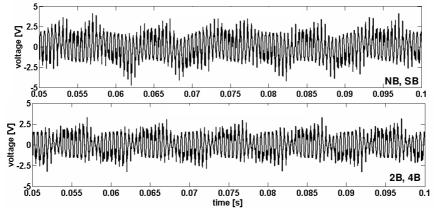
Fig. 5.3.18.a Time-domain representation of the voltages induced in search coil "p-1" – static eccentricity – simulations at half load.
