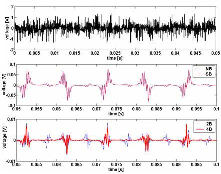
Fig. 5.2.19 Time-domain representation of the voltages induced in the search coil placed around two pole pitches -3 broken rotor bars - measurements (topmost figure) and simulations taken at half load.
