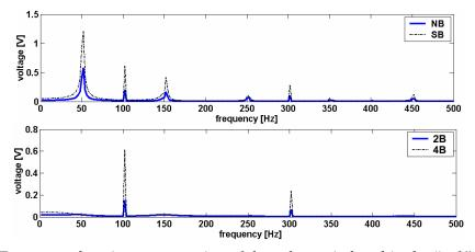
*Fig. 5.2.8 Frequency-domain representation of the voltages induced in the "p-1" search coil* – *inter-turn short circuit* – *simulations at half load.*
