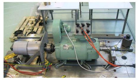
Fig. 4.6 Test induction motor (left) and DC generator used as load.
