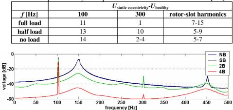
Fig. 5.3.14 Frequency-domain representation of the voltage induced in the "p+1" search coil – static eccentricity – simulations at half load.
