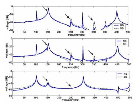
Fig. 5.2.13 Characteristic frequency sidebands produced by the inter-turn short circuit in the indications provided by "p+1" search coil – simulations at full load (topmost figure), half load (middle figure), and no load (bottom figure).
