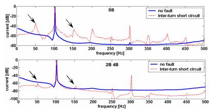
*Fig. 5.1.1 Frequency spectrum of the branch current – inter-turn short circuit – simulations at full load.*
