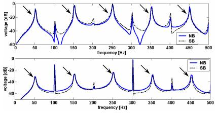
Fig. 5.2.6 Frequency-domain representation of the voltages induced in the search coil wound around two pole pitches – inter-turn short circuit – simulations at full load (top) and no load (bottom).
