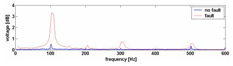
*Fig. 5.2.15 Frequency-domain representation of the voltage induced during the inter-turn short circuit in the search coil positioned around the motor shaft – measurements at half load.*
