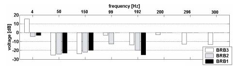
Fig. 5.2.30 Characteristic frequency sidebands produced by a rotor cage-related fault in the indications provided by the search coil placed at the non-drive end of the motor – measurements at full load.
