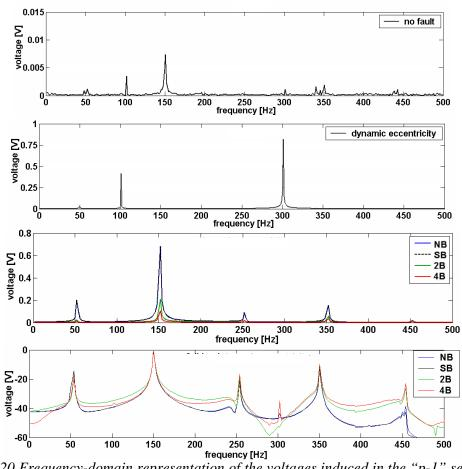
Fig. 5.3.20 Frequency-domain representation of the voltages induced in the "p-1" search coil – healthy and dynamic eccentricity – measurements (two topmost figures) and simulations at full load.
