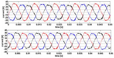
*Fig. 5.1.2 Stator winding branch currents – inter-turn short circuit (top) and no fault (bottom) – measurements at half load.*
