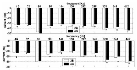
Fig. 5.1.5 Characteristic fault frequencies produced by rotor cage-related faults in the stator winding branch current spectrum - simulations (represented by bars) and measurements (represented by dots) at full load. One broken rotor bar (top) and three broken rotor bars (bottom).
