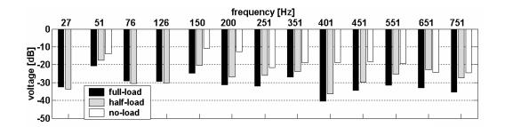
Fig. 5.3.28 Characteristic frequency sideband components produced by the dynamic eccentricity in the indications provided by the search coil placed at the non-drive end of the motor – measurements at various loads.
