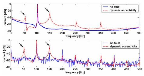
Fig. 5.1.6 Spectrum content of the stator winding branch current – dynamic eccentricity – simulations (top) and measurements (bottom) at half load. Figure corresponding to the operation of a motor equipped with the original stator winding configuration of type "2B".
