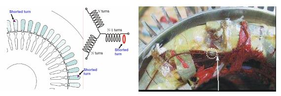
Fig. 4.1 Description of the turn-to-turn short circuit implemented in the simulations (left figure) and measurements (right figure).
