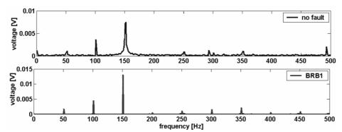
*Fig. 5.2.25.b Frequency-domain representation of the voltages induced in the "p-1" search coil – measurements at no load.*
