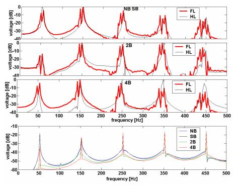
*Fig. 5.2.20 Frequency-domain representation of the voltages induced in the search coil wound around two pole pitches – 3 broken rotor bars – simulations at full load and half load (topmost three figures) and no load (bottom figure).*
