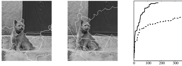
Figure 3.5: Data driven vs. random proposals. Left: result of data driven segmentation after 179 samples. Center: result of segmentation using random proposal distributions in the same amount of CPU time (365 samples). Metropolis-Hastings acceptance probabilities were 27 % and 20 %, respectively. Right: evolution of log posterior probabilities \log p(\mathbf{S}|\mathbf{I}, M) in the MCMC chains with data driven ( continuous ) and random ( dashed ) proposal distributions.
