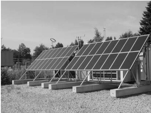
Figure 5.1: 32 CdTe and CIGS modules under measurement at the HUT test site in July 2002.
