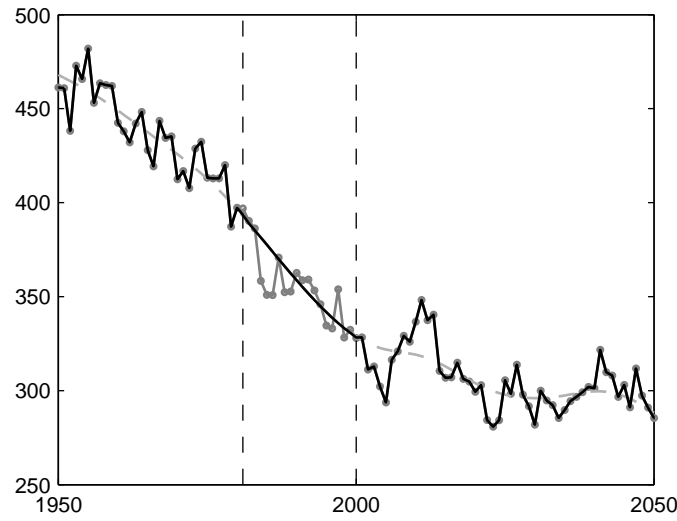
Figure 4.30: The original prediction over missing data at 1981 – 2000. The gray line is the true signal, the dashed line is the long term prediction result, and the black line is the combined long and short term prediction result.
