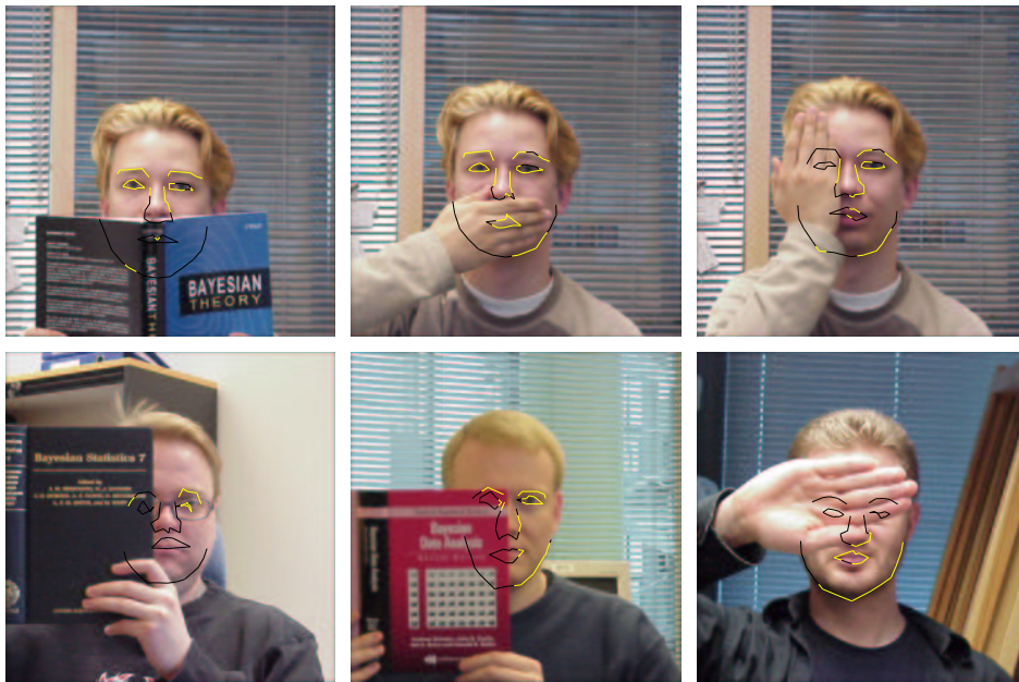
Figure 6.6: Matching results for images with real occlusions. The graphs show the sample means. The dark portions of the graphs denote features with detection probabilities below 0.5, and the light portions features with detection probabilities above 0.5. The results are promising: most features are matched correctly, although there are errors both in the locations of the features as well as their detection statuses.
