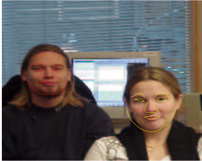
Figure 6.11: Matching with multiple object instances using the multiple object model, real image. The yellow graph represents the sample mean of the first run of the sampler, and the red graph the sample mean of the second run of the sampler with the area around the first mean marked occluded. The number of effectively detected features was approximately 46 after both runs. After a third run this value dropped to 11.
