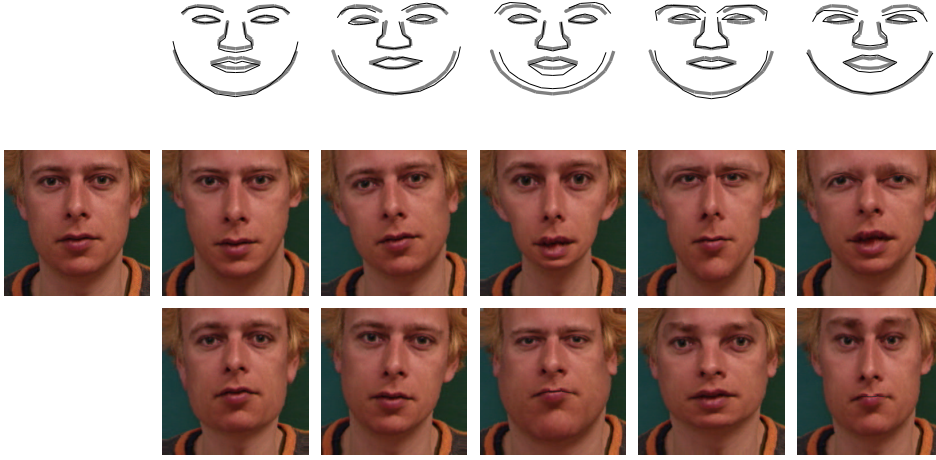
Figure 4.2: Principal component shape model. In the upper row, the thick gray graphs show the mean shape and the thinner black graphs the leading eigenvectors added to the mean. In the other rows, the face on the left has been morphed according to the principal components, both in the positive (middle row) and negative (lower row) directions. Components 1 and 2 appear to be related to rotations, while components 3, 4, and 5 are shape-related.
