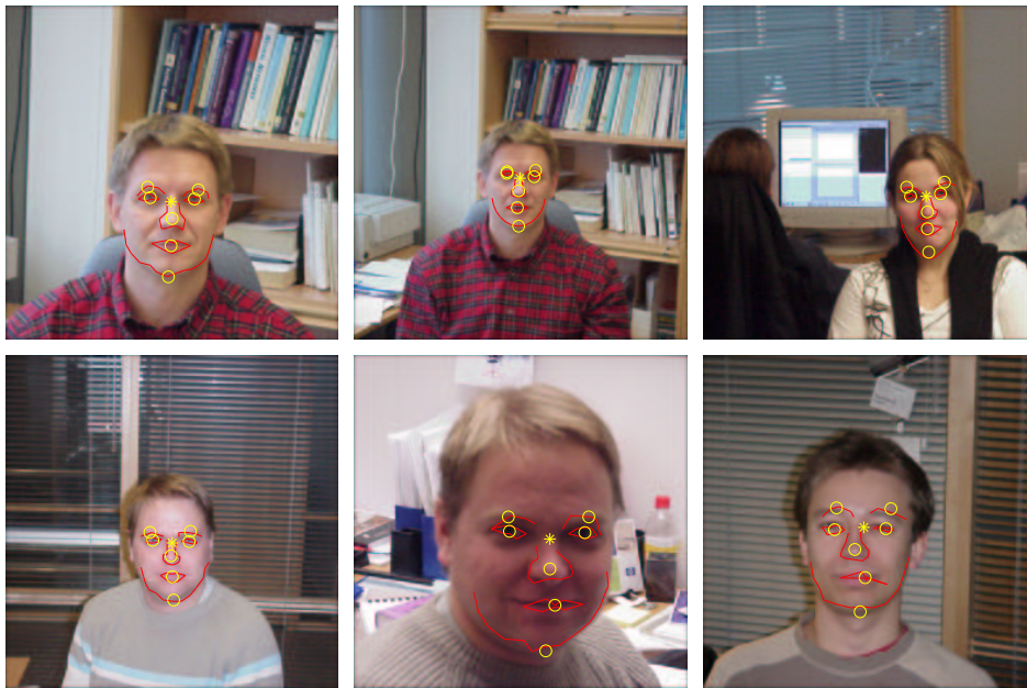
Figure 6.8: A set of matched objects in real-world conditions. Again, the shown graphs are obtained using the base resolution with the largest number of effectively detected features.
