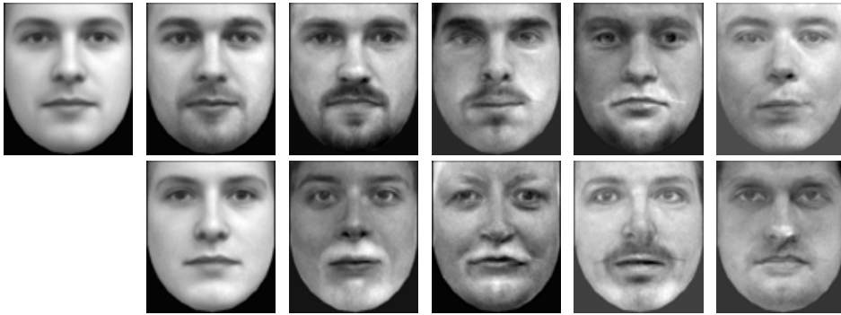
Figure 3.12: Examples of Eigenfaces. Training image shapes from the IMM-DTU database (Stegmann, 2002) were normalized and backgrounds eliminated. The first image on the left shows the mean texture and the following 5 columns depict the sum of the mean shape and the first five principal components, with positive coefficients in the top row and negative coefficients in the bottom row.
