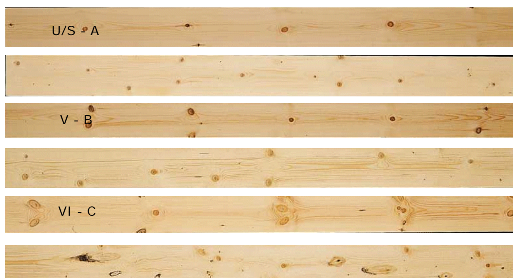
Figure 6. Three sawnwood quality classes U/S-A (above pine, below spruce), V-B (middle p, s), VI-C (below p, s) according to Nordic timber (1994).
