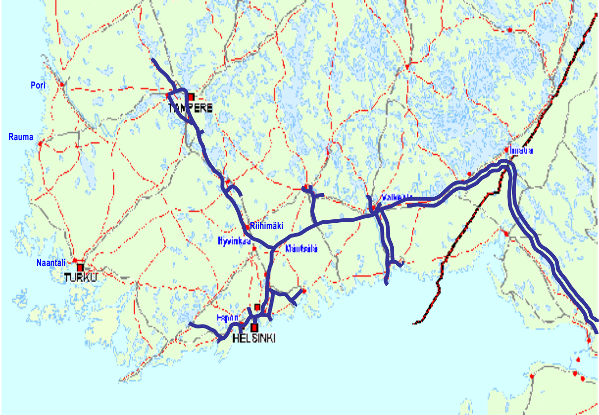
Figure 2.5 The Finnish natural gas pipeline transmission system.
