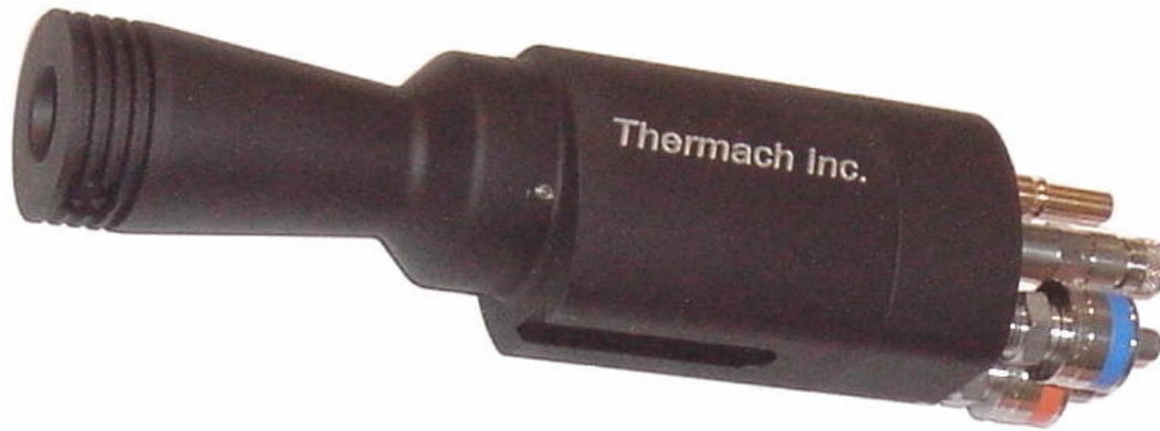
Figure 3. Miller Thermal HV-2000 HVOF spray gun.
