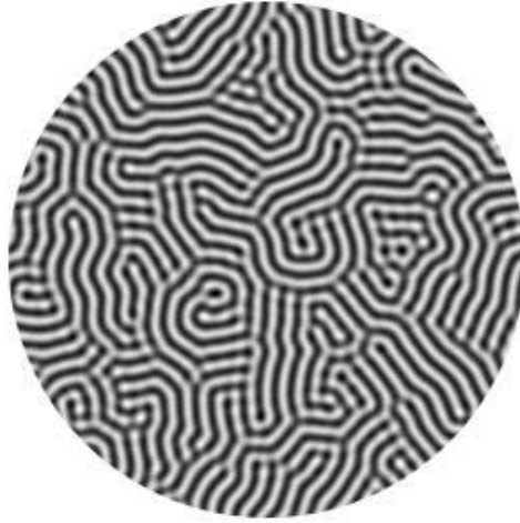
Figure 2.6: Computer simulation of Rayleigh-Bénard convection using the Swift-Hohenberg model. The view is from above. Notice that the convective cells are not ordered as in the ideal situation of Figure 2.5. The dark and light colors denote the domains with upward movement (warmer sparse liquid) and downward movement (cooler dense liquid), respectively. (Image: Mikko Karttunen, Helsinki University of Technology.)
