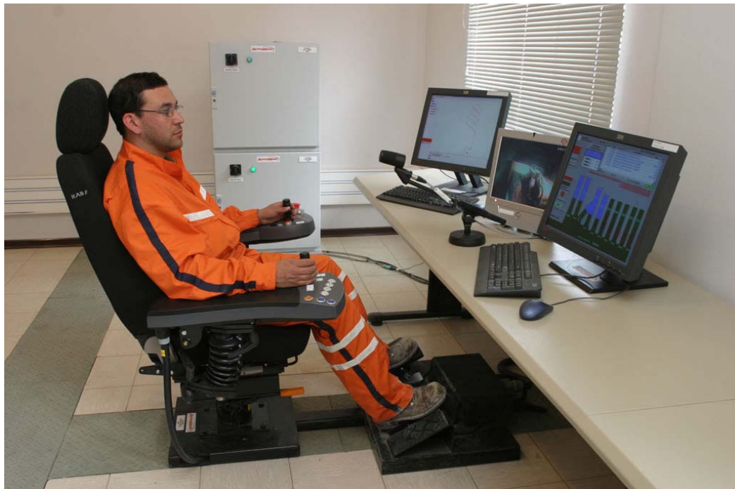
Figure 3: The final operator station for the LHD control presented in Paper II. The control interface (joysticks and buttons in the chair are very similar to a manual machine). – Figure provided by Sandvik Tamrock
