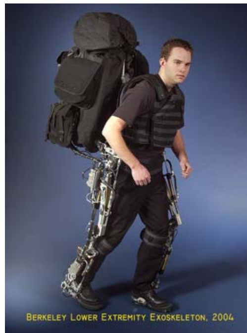
Figure 10: Power assistant exoskeleton, adopted from [Berkeley]
