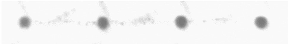
Figure 5.42. The output of the 1×4 power splitter recorded with an IR camera.
