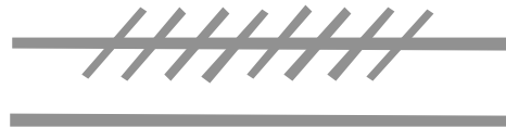
Figure 5.33. Schematic representation of the test layout for measuring the excess loss, and degradation of the PER due to a waveguide crossing at different angles. The test waveguide had 60 dummy crossings. Transmission of the intersected waveguide was referenced to a continuous waveguide along side it.
