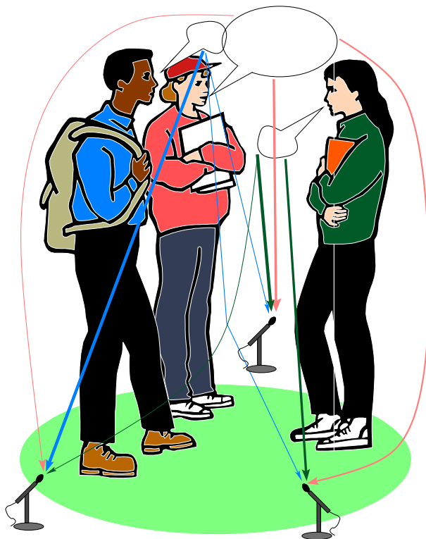
Figure 1.1: A MIMO system. Three signals produced by sources (speakers) are recorded by three sensors (microphones). Each microphone records slightly different mixture of speech due to the differences in the relative distances and angles between the mouths and the microphones, and due to the multipath propagation, i.e. the same waveform propagates via different paths.
