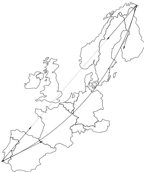
Figure 2.1: The shortest path between Vardø, Norway, and Sagres, Portugal, on the map (dotted line) and in reality (solid arc). The gradients towards the shortest path are given using the map geometry (Euclidean) and the true geometry (Riemannian).
