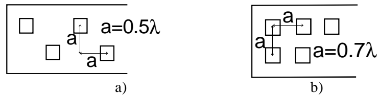
Figure 16. a) Zigzag antenna array used indoors. b) Linear antenna array used outdoors.
