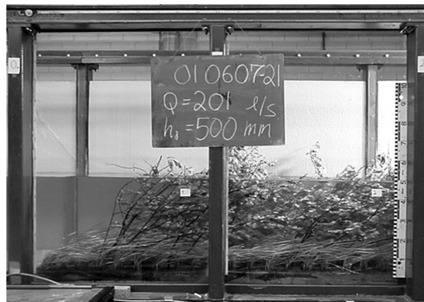
Figure 3. Test run 010607-21 of series S3Pa with leafy willows and sedges. The average flow velocity was 38.7 cm/s.
