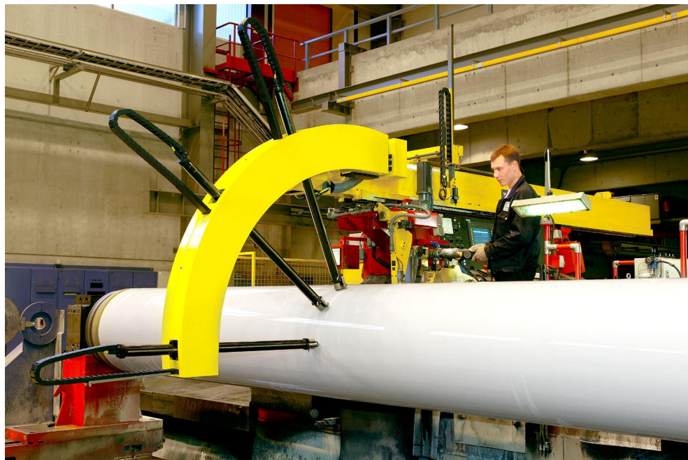
Figure 15 Modernised roll grinding machine of Fortek Oy. The machine is situated at the Stora Enso Corp. Oulu Paper Mill. The control system includes 3D grinding control technology. The fully-automatic 3D measuring device is based on the four-point measuring method.
