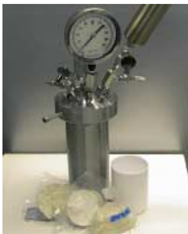
Figure 4-3. Experimental set-up for (PO) bleaching studies. The pulp samples and the teflon mug are shown. The kappa numbers of the samples shown are from the left 7, 4, and 10.
